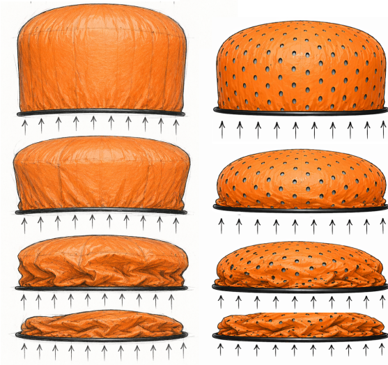
Figure 6. Sketch of bag inflation setup without (left) and with (right) openings.
