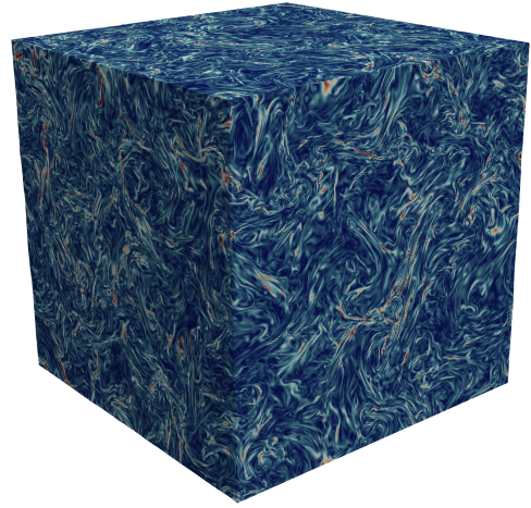
Figure 1. Visualisation of the magnitude of the vorticity field \omega = \nabla \times \mathbf{u} from numerical simulations of magnetohydrodynamic turbulence (Capocci et al. , 2025a).
