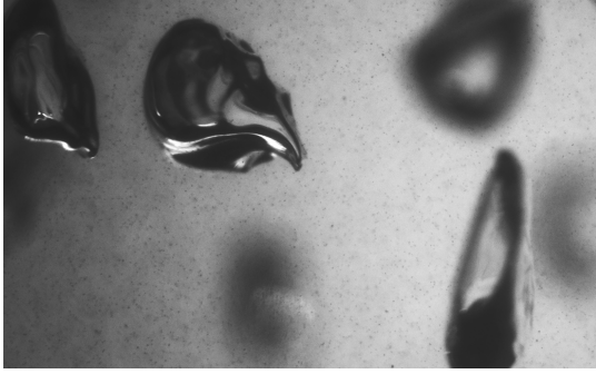
Figure 8. Cropped snapshot showing simultaneous imaging of tracer shadows and bubble interfaces.
