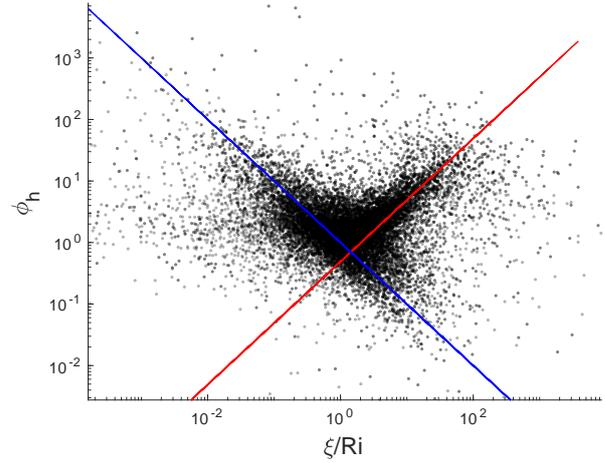
Figure 4. Non-dimensional buoyancy gradient as a function of the parameter  $\xi/Ri$ .
