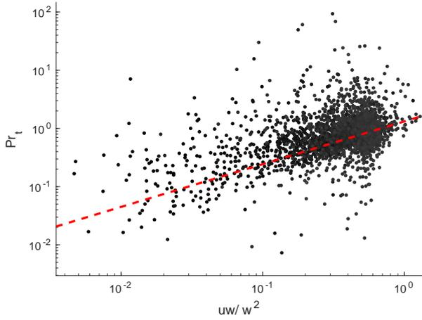
Figure 2. Turbulent Prandtl number as a function of  $\overline{uw}/\overline{w^2}$  for data with  $\xi > 0.2$ . Red line is the best-fit power-law function (30).
