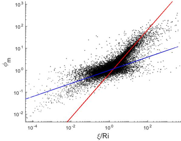
Figure 3. Non-dimensional wind velocity gradient as a function of the parameter  $\xi/Ri$ .
