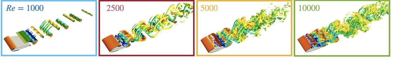
Figure 1. Instantaneous spanwise periodic flow around a NACA0012 airfoil at \alpha = 14^\circ and different Reynolds numbers. Flow field visualized with isocontour of Q-criterion colored by streamwise velocity.
