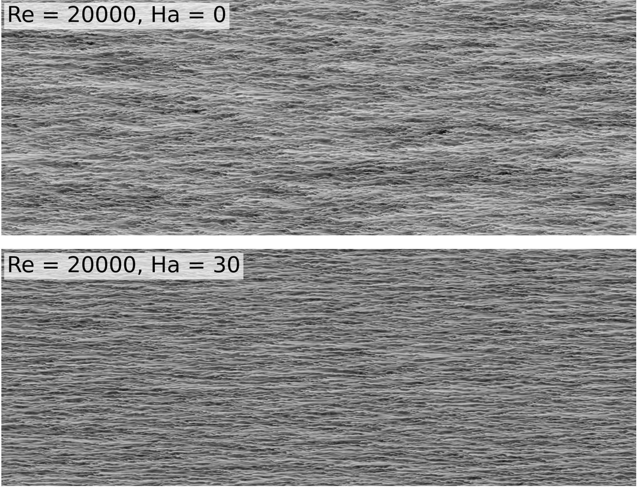
Figure 3. Streamwise velocity at where  $\langle u'^2 \rangle$  is maximum
