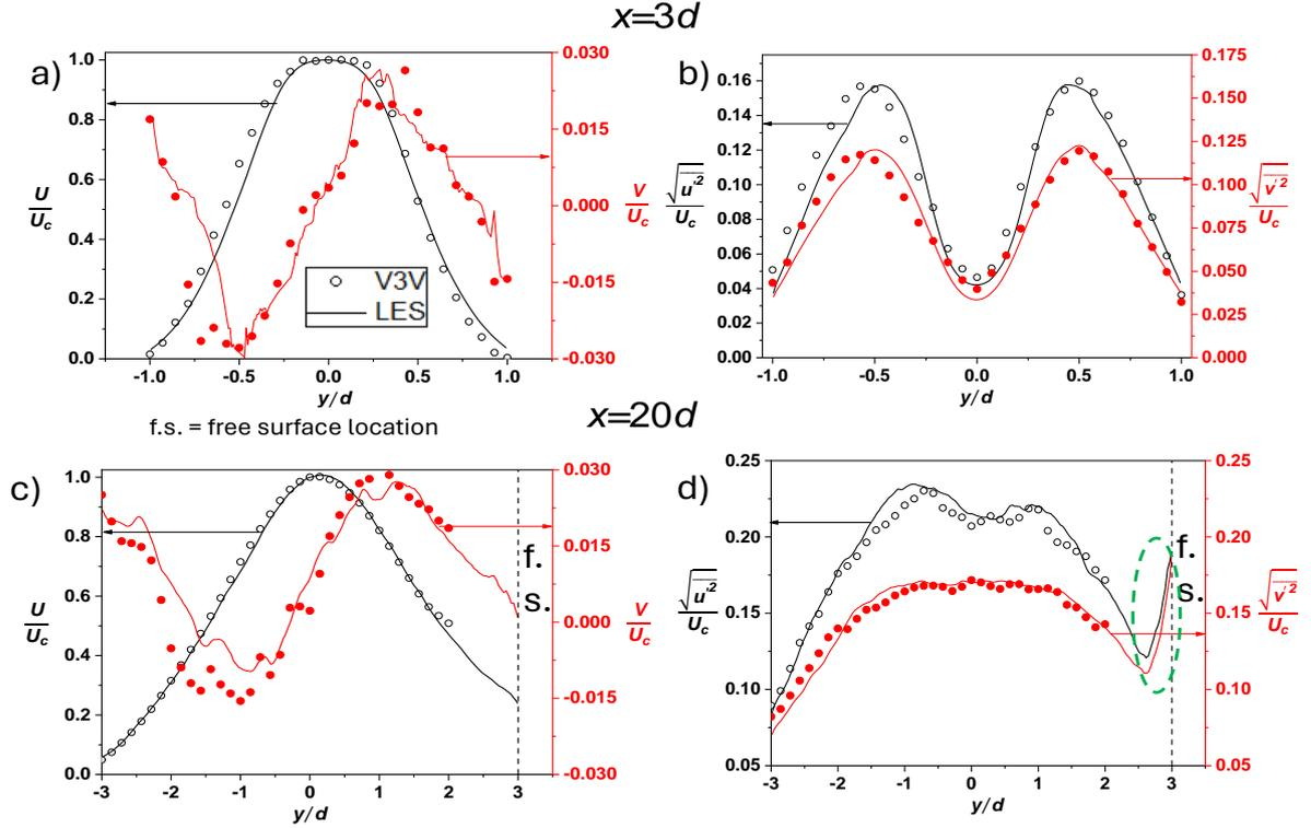
Figure 2. Experimental and numerical data comparison in the near field and far field of the jet. The circle symbol denotes V3V data, and the line represents LES data. The dotted vertical line describes the position of the free surface location.
