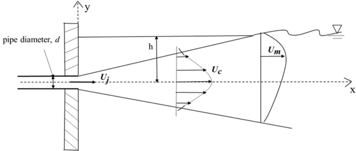
Figure 1. Surface jet schematic describing all the important parameters which defines a surface jet
