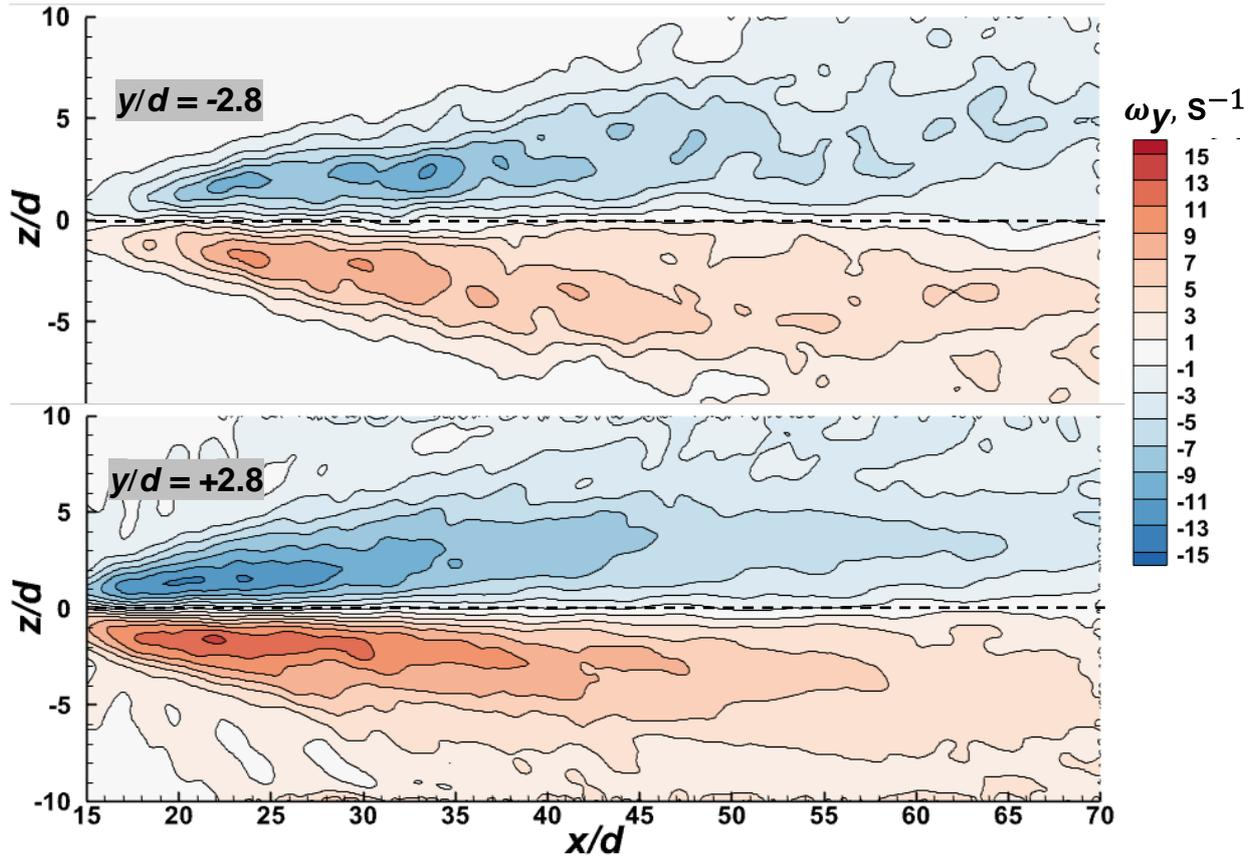
Figure 4. Comparison of mean y-vorticity on a plane parallel to the free surface and located at two different radial positions: closer and away from the free surface.
