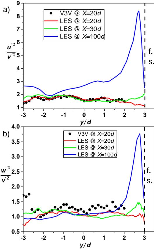
Figure 3. Ratios between square of turbulence fluctuations in the directions parallel to the free surface and perpendicular to the free surface at different axial locations of the jet
