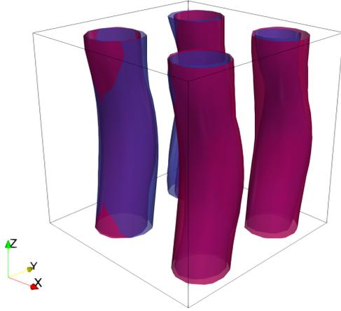
Figure 2. Visualization of the reconstructed vorticity field by CNN-AE (isosurfaces of  $|\omega_3^>|^2$ ). The blue and red isosurfaces are the true and reconstructed vorticity fields, respectively. Here, the threshold is chosen as  $m_q + 2\sigma_q$ , where  $m_q$  and  $\sigma_q$  are the mean and standard deviation of  $|\omega_3^>|^2$ , respectively.
