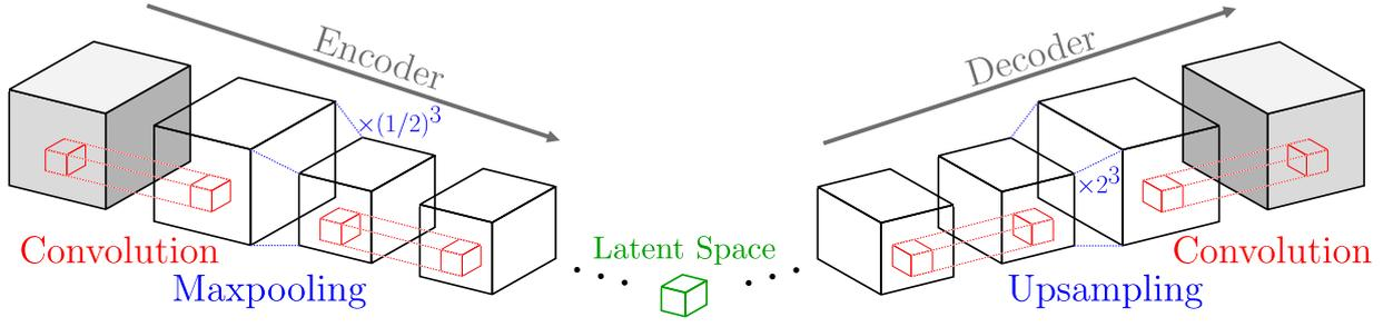
Figure 1. Schematic of CNN-AE structure. CNN-AE has two parts: an encoder and a decoder. The encoder consists of a convolution layer and a pooling layer connected alternately and reduces the input dimension. In the present study, we reduce the input dimension to 8. The decoder consists of a convolution layer and an upsampling layer connected alternately, which expands the latent dimension to the input dimension.
