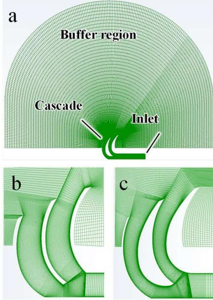
Figure 1. Computational mesh of (a) whole domain, vicinity of cascade of (b) original model and (c) filled model.
