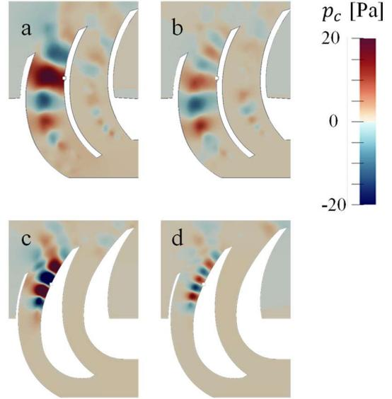
Figure 6. Conditionally averaged pressure  $p_c$  of the original model (a, b) and the filled model (c, d). Reference signals are  $F_a$  for (a) and (c), and  $F_b$  for (b) and (d). Condition is “reference signal takes positive peak values”.
