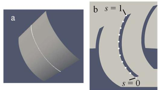
Figure 4. (a) sampling line on the suction surface. (b) definition of  $s$ .
