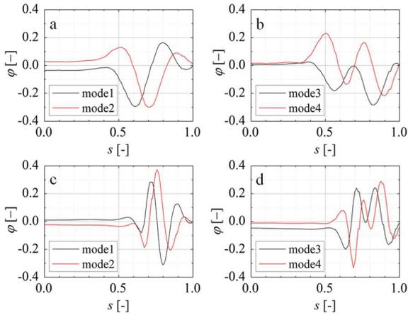
Figure 5. POD modes of fluctuating pressure on the suction surface. (a) modes 1, 2 and (b) modes 3, 4 of the original model. (c) modes 1, 2 and (d) modes 3, 4 of the filled model.
