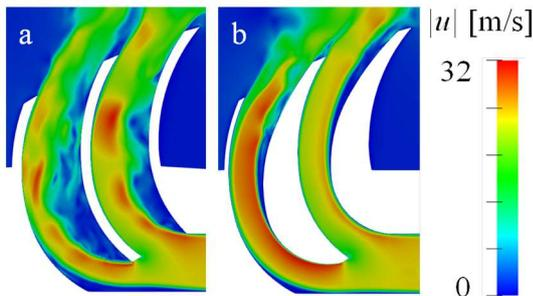
Figure 2. Instantaneous value of magnitude of velocity of (a) original model and (b) filled model.
