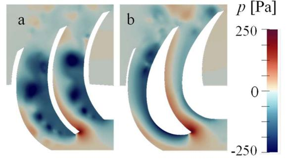
Figure 3. Instantaneous value of pressure of (a) original model and (b) filled model.
