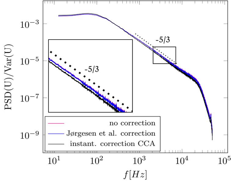
Figure 6. Velocity spectra at 55 m/s taken in correspondence of the  $\sigma_U$  peak, effect of the sensitivity correction.
