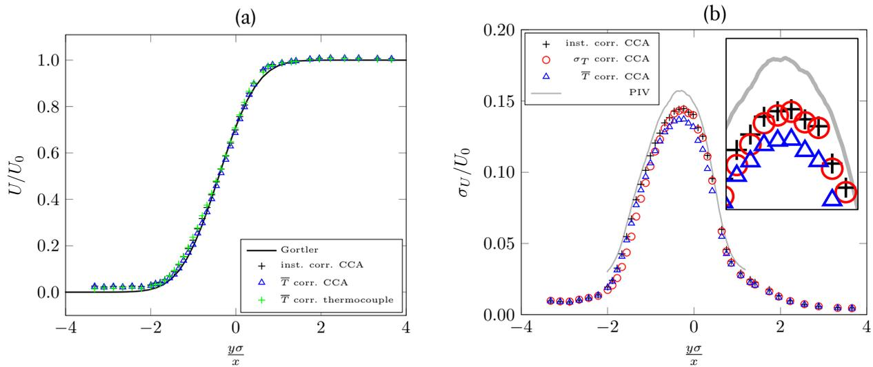
Figure 7. Mean (a) and standard deviation (b) streamwise velocity profiles, comparison between instantaneous correction and correction using the statistics of temperature profiles.
