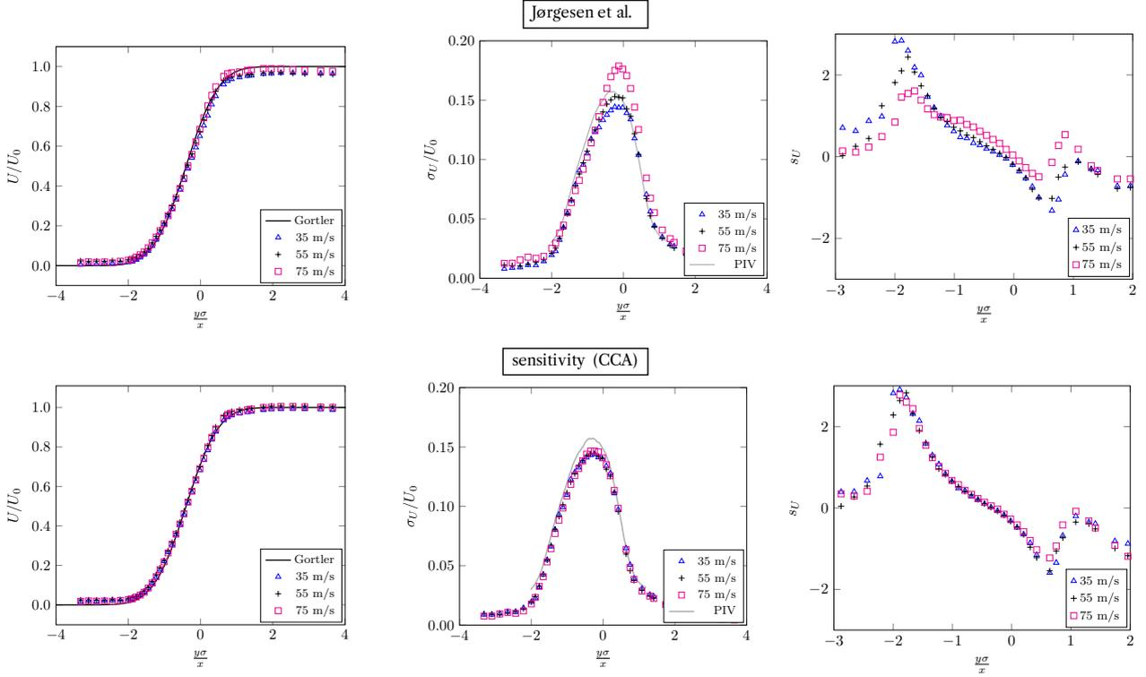
Figure 5. Mean velocity  $U/U_0$ , standard deviation  $\sigma_U/U_0$  and skewness profiles. Effect of the free-stream condition  $U_0$ . Reference value of  $U_0$  obtained with pitot used to normalise the profiles.
