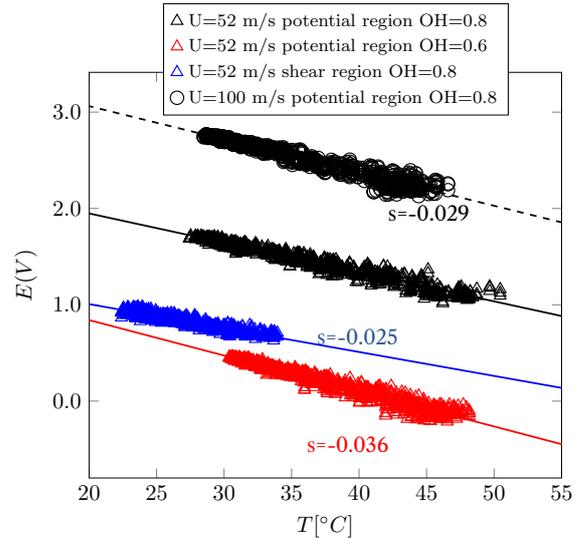
Figure 3. Temperature sensitivity evaluation for several velocities, effect of velocity, over-heat ratio and position, temperature data obtained with the CCA cold wire.
