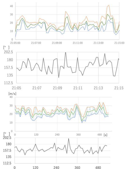
Figure 11. Time series of horizontal wind speed and direction of Case 1. Simulation result (top), observational data (bottom). Orange and blue lines show the 3-s maximum and minimum in 10 s of evaluation time. Dark gray lines 10-s averaged wind direction.
