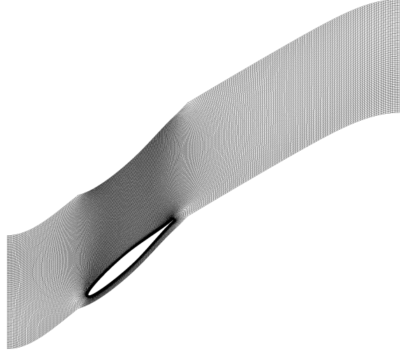
Figure 8. Mesh used for NACA 65-010 compressor cascade case
