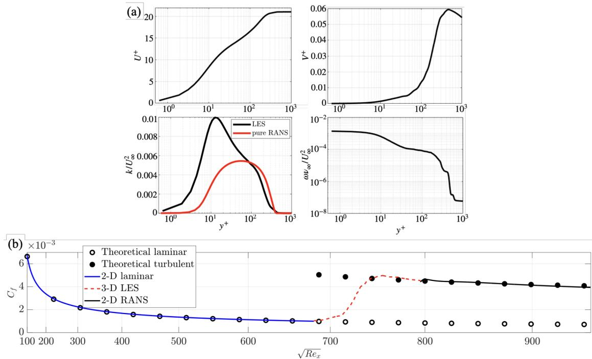
Figure 4. Selected computational results from the modified RANS inlet: (a) The mean velocity ( $U^+$  and  $V^+$ ) and turbulence quantities ( $k$  and  $\omega$ ) assigned at RANS inlet. (b) Averaged skin friction coefficient  $C_f$ .
