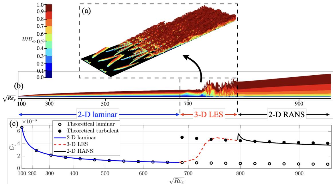
Figure 3. Selected computational results: (a) Vortical structures visualization using iso-surface of  $Q = 20$  coloured by normalized streamwise velocity in the LES domain. (b) Normalized instantaneous streamwise velocity fields on a spanwise-normal plane; the scale  $x:y=1:6$  is used for the visualization purpose. (c) Averaged skin friction coefficient  $C_f$ .
