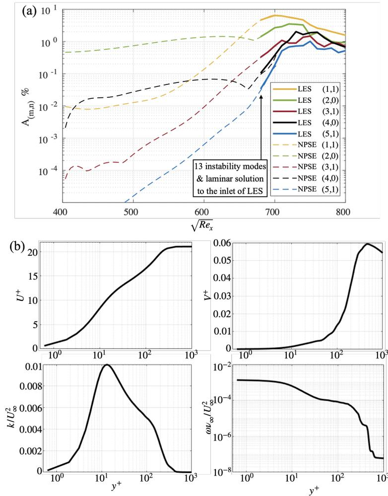
Figure 2. Computational data for (a) NPSE-LES and (b) LES-RANS interfaces: (a) amplitude growth of 5 major modes from NPSE analysis among 13 instabilities assigned at the LES inlet (b) mean velocity ( $U^+$  and  $V^+$ ) and turbulence quantities ( $k$  and  $\omega$ ) assigned at RANS inlet from the LES computation.
