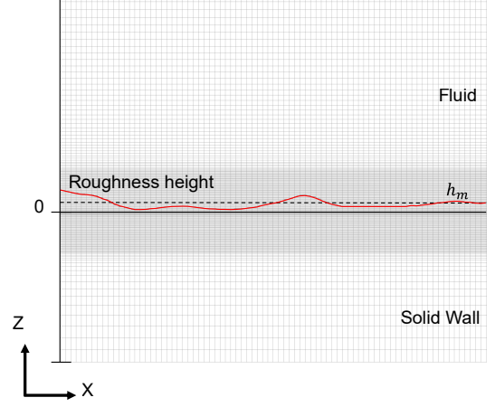
Figure 2. Mask function shape and Grid resolution near the wall.
