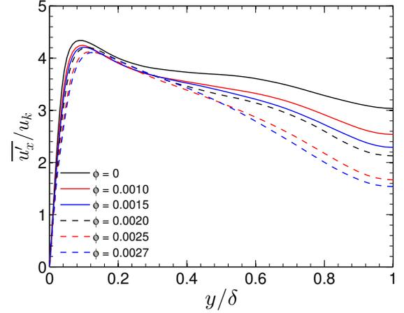
Figure 5: The ratio of streamwise root mean square fluctuations ( $u'_x$ ) and Kolmogorov velocity scale ( $\eta$ ) plotted in the wall-normal direction for a range of volume fractions for  $St = 210.93$ .
