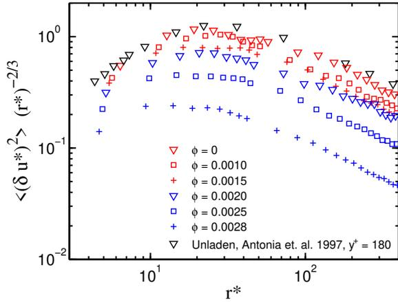
Figure 3: The second-order velocity structure-functions multiplied with  $r^{*-2/3}$  for different volume fractions at channel center location ( $y^+ = 180$ ) with  $St = 210.93$ .
