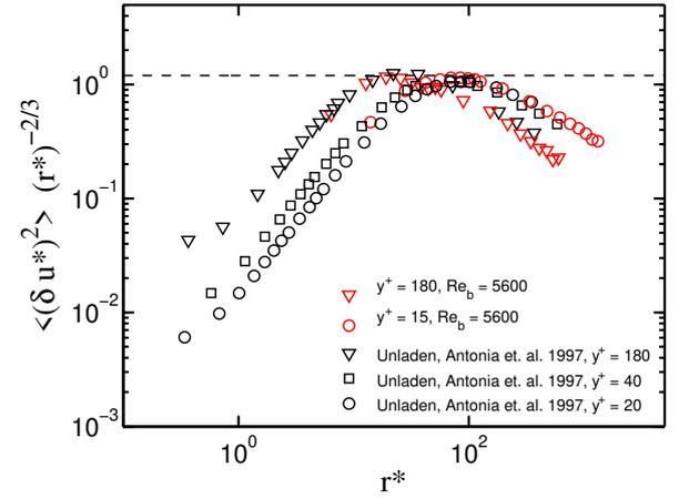
Figure 2: The second-order velocity structure-functions multiplied with  $r^{*-2/3}$  for unladen cases. The dashed line is plotted at 1.2.
