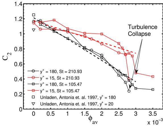
Figure 4: The peak of second-order velocity structure-function plotted for different volume fractions. The dashed lines are the fitting curves.
