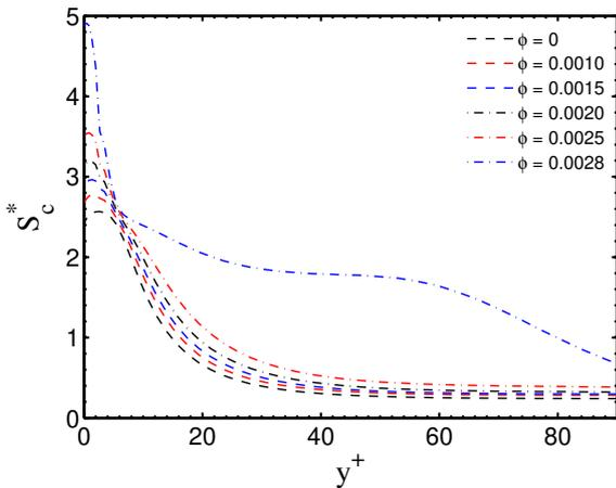
Figure 1: The ratio of Kolmogorov time scale to mean shear time scale for different volume fractions at  $St = 210.93$ .
