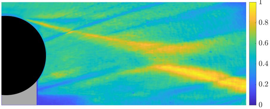
(b) Map of the normalized standard deviation of temporal fluctuations in schlieren intensity.
