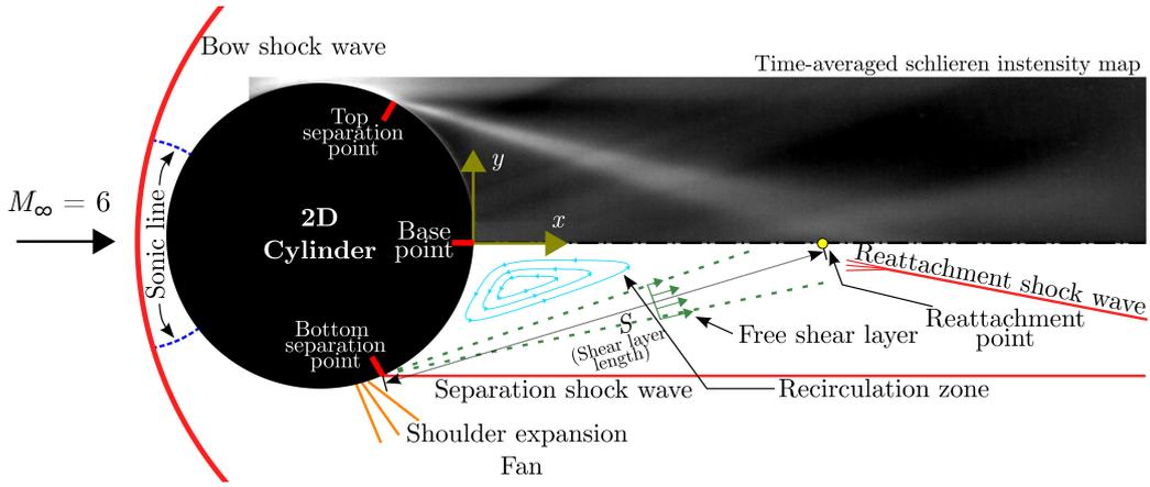
Figure 1: Key features of hypersonic flow past a 2D circular cylinder. The time-averaged schlieren intensity map, which was experimentally obtained, indicates density gradients in the direction normal to the free-stream flow.
