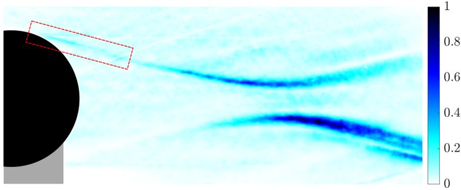
Figure 4: Amplitude map of SPOD mode 1. The red-colored bounding box highlights the upstream portion of the shear layer where a signature of energetic activity is visible.
