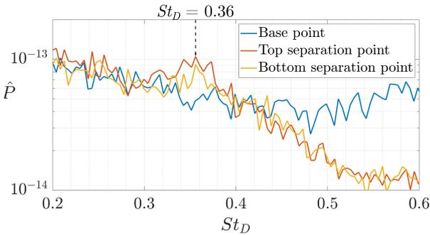
Figure 5: Power spectral density ( $\hat{P}$ ) of non-dimensional pressure ( $p/P_0$ ) fluctuations at the top and bottom separation points and the base point.
