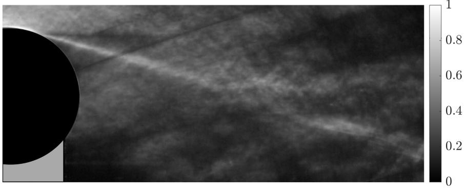
(a) An instantaneous schlieren snapshot with normalized intensity, which indicates density gradients in the direction normal to the free-stream flow.
