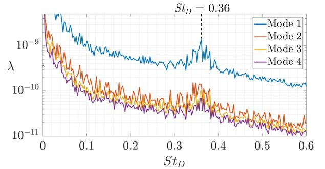
Figure 3: The modal energy spectrum of the first four modes obtained from SPOD. The dominant frequency corresponding to the oscillations can be identified as  $St_D = 0.36$ .
