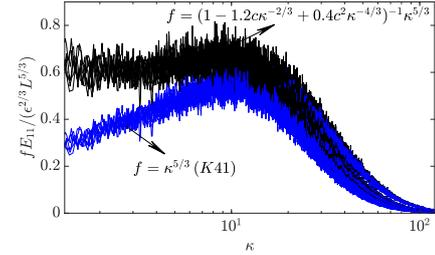
Figure 4. Validation of expression 8 using hot wire anemometry. The compensated spectra become flat using the out-of-equilibrium correction, and not the classical K41 formulation.
