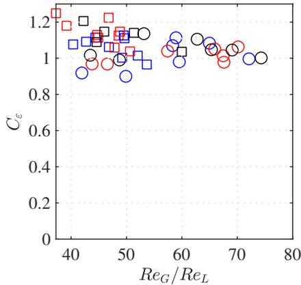
Figure 5. Measured dissipation coefficient for the two grids tested (circles and squares) for inlet velocities of 7, 5 and 4  $\text{ms}^{-1}$  (blue, red and black colours).
