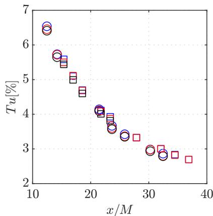
Figure 6. Measured turbulence intensities for the two grids tested (circles and squares) for inlet velocities of 7, 5 and 4  $\text{ms}^{-1}$  (blue, red and black colours).
