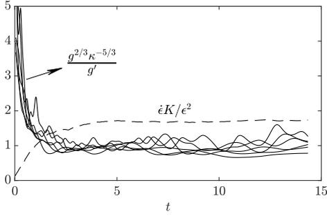
Figure 2. Evolution of the two sides of equation 5 over time, using the DNS dataset (forcing stops at  $t = 0$ ).  $g^{2/3} \kappa^{-5/3} / g'$  (solid lines) is plotted for  $\kappa = 3, 4, 5, 6, 7, 8, 10$ .
