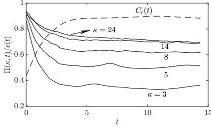
Figure 1.  $g \equiv \Pi/\varepsilon$  (solid lines) and  $C_\varepsilon$  (dashed line) as a function of time, in decaying periodic box turbulence.  $t = 0$  marks the onset of decay. Note that  $\kappa = kL$ .
