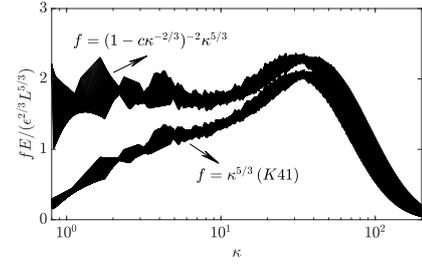
Figure 3. Validation of expression 7 using DNS. The compensated spectra become flat using the out-of-equilibrium correction, and not the classical K41 formulation.
