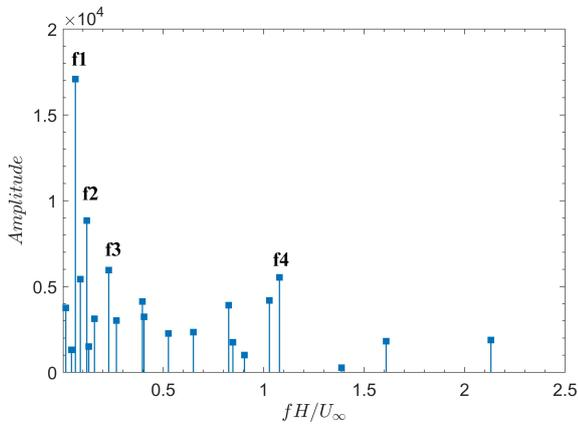
Figure 2. Amplitudes of difference modes for adiabatic wall.
