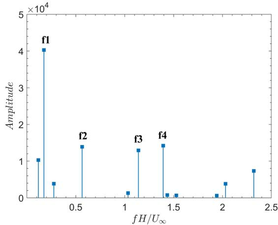
Figure 4. Amplitudes of difference modes for heated wall.
