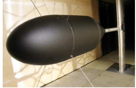
Figure 2: BOR installed in the Stability Wind Tunnel Kevlar-walled anechoic test section, including supporting tethers, sting, and mounting post.
