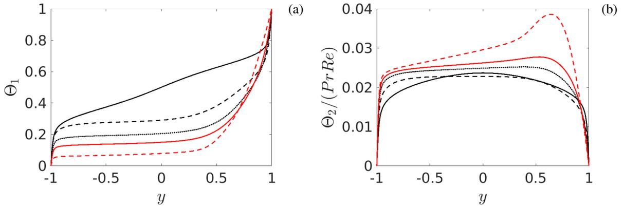
Figure 2. Mean scalar profiles (a) in the case with the assigned scalar difference at the walls and (b) the case with the constant mean streamwise scalar gradient at  $Ro = 0$  (black solid),  $Ro = 0.15$  (black dashed),  $Ro = 0.3$  (black dotted),  $Ro = 0.45$  (red solid),  $Ro = 0.75$  (red dashed).
