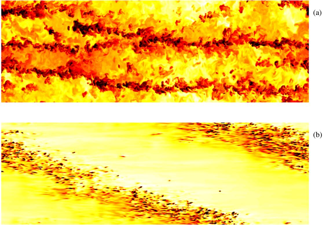
Figure 1. Visualizations of (a) the scalar field in an  $x$ - $z$  plane on the unstable side at  $y = -0.5$  at  $Ro = 0.15$  and (b) of the scalar gradient at the wall at  $y = 1$  on the stable side at  $Ro = 0.45$ .
