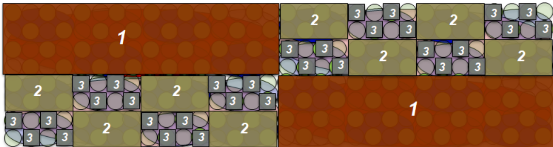
Figure 8. Schematic of the apportioning of the signature of aggregated scales on a wall-parallel plane, showing the scaling of Equation 11. Numbers denote the signature of a structure centered at y_m .
