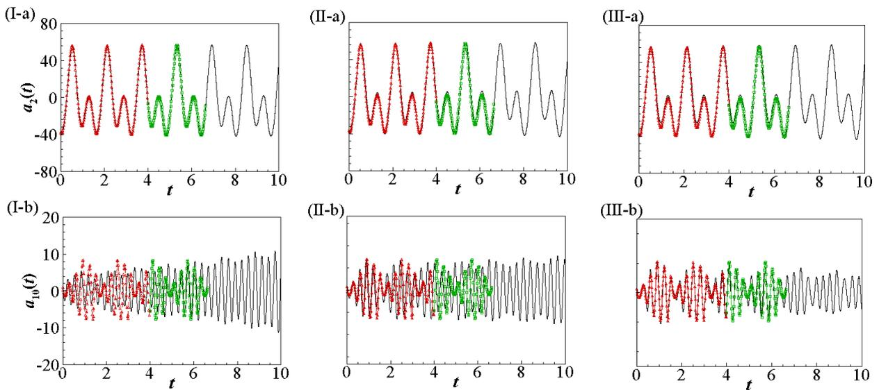
Fig. 5 Temporal coefficients of mode 2 (a) and mode 10 (b), with 11 (I), 15 (II) and 21 (III) modes. —△— projected DNS data in the time range that POD and DMD is performed, —□— beyond the time range that POD and DMD is performed, — ROM
