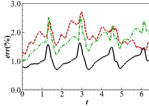
Fig. 6 Error of ROMs. Red dashed line: 11 modes; green dashed-dot line: 15 modes; black solid line: 21 modes
