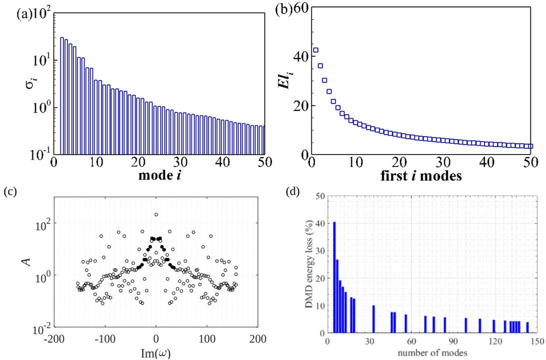
Fig. 3 Energy of POD modes (a), total energy loss of the first  $i$  modes (b), DMD frequency spectrum (c) and energy loss of a certain number of modes (d), solid circles in (c) are modes selected by SP algorithm
