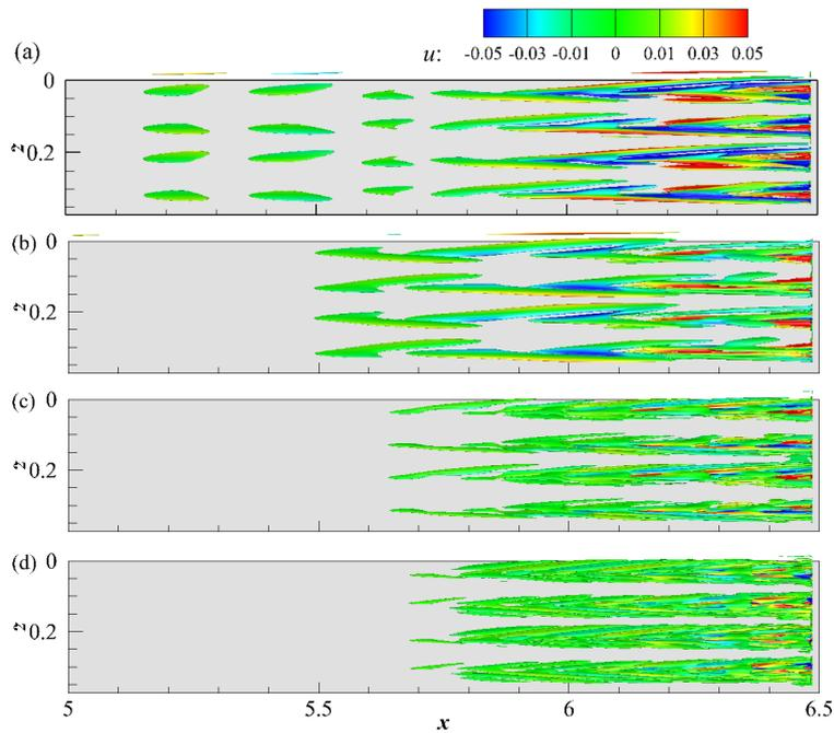
Fig.4 Iso-surfaces of  $Q=0.0001$  colored by  $u$ . (a-d) mode 2, 4, 6, and 8 respectively.
