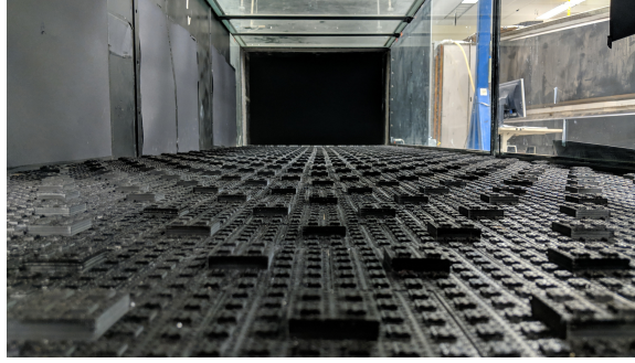
Figure 2: Photograph of the multifractal roughness array in the wind tunnel.
