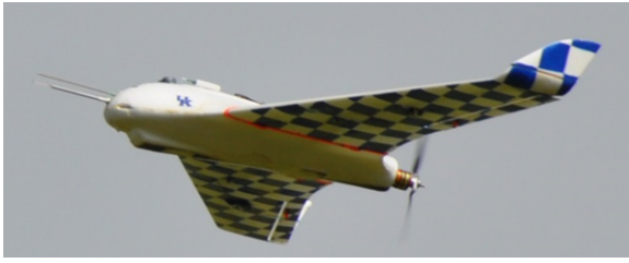
Figure 1. Modified Skywalker X8 airframe used for turbulence measurements.
