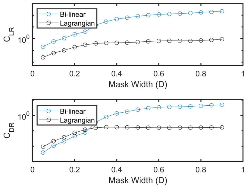
Figure 5. Mean % error in estimation of lift (a) and drag (b) coefficients employing the standard impulse formulation using the Lagrangian interpolation scheme and Bi-linear interpolation.
