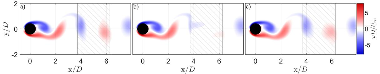
Figure 3. A CFD data set where a mask is artificially applied to the hatched grey region. (a) is the original field, (b) is the recreation using linear interpolation, and (c) is the recreation using the Lagrangian interpolation scheme
