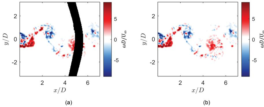
Figure 2. Raw masked (a) and unmasked (b) vorticity fields from experimental PIV data highlighting the output of the Lagrangian interpolation algorithm.
