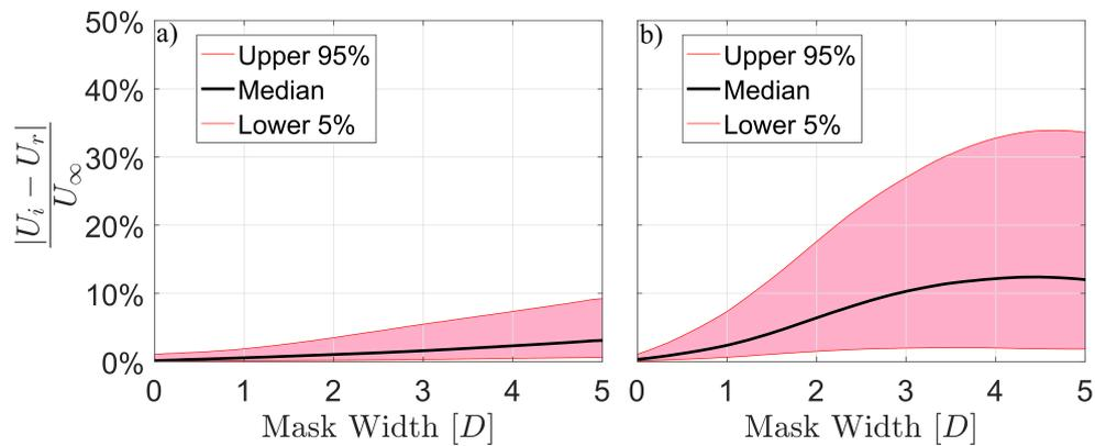
Figure 4. Median, 95%, and 5% absolute relative velocity error of reconstructed fields in the region  $\Pi_m$  using the Lagrangian interpolation scheme (a) and linear interpolation (b).
