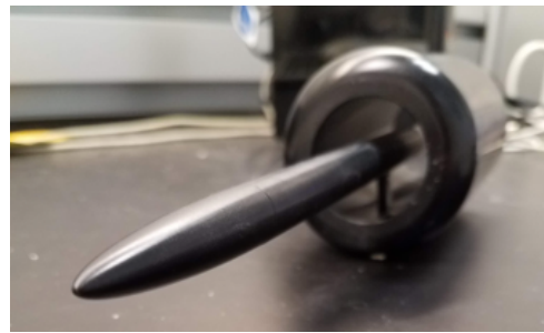
Figure 2: The body of rotation is shown outside of the experimental pipe. The sting supporting the body can be observed.
