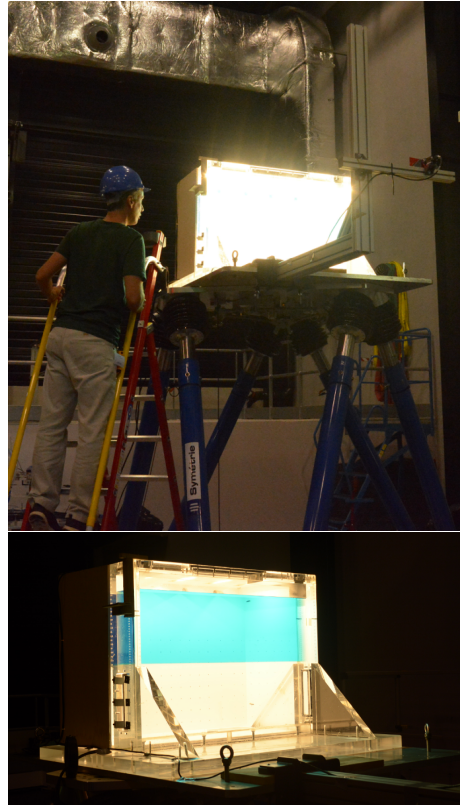
Figure 1. Experimental setup. Top : general view of the platform on the hexapod. The experimental tank is empty, and enlightened from the back by a LED panel. The arm holding the camera is visible. Bottom : experimental tank filled with two layer miscible fluid, before the experiment. Note the initial sharpness of the interface. Blue dye is added in the fresh layer for measurement.
