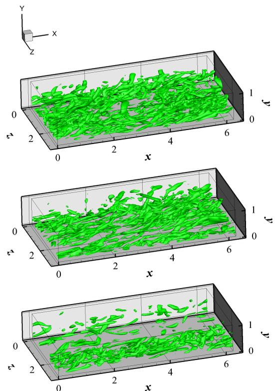
Fig.4. Distributions of vortex structures via the Q-criterion ( $Q=2.0$ ): (a)  $Da = 10^{-4}$ ,  $\varphi = 0.9$ , (b)  $Da = 10^{-4}$ ,  $\varphi = 0.5$  (c)  $Da = 10^{-5}$ ,  $\varphi = 0.7$ .
