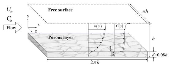
Fig. 1. Sketch of DO transfer to permeable microbial sediment bed.
