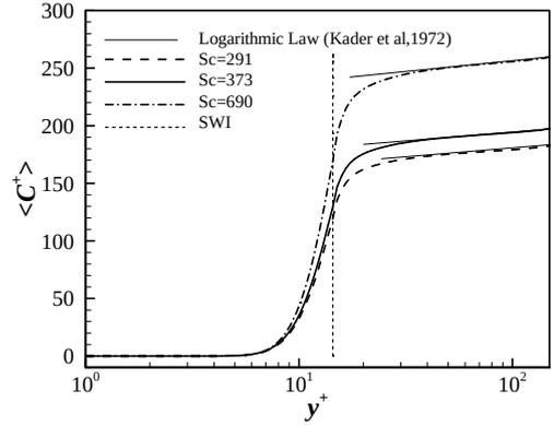
Fig. 5. Distributions of DO mean concentration, at different Schmidt numbers.
