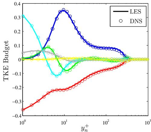
Figure 7: Comparison of turbulent kinetic energy budget for a NACA4412 wing section at the suction side location of  $x/c = 0.7$ . The circles represent DNS data from Hosseini *et al.* (2016) while the lines are data from the LES. The individual terms are color coded as: **Production**, **Dissipation**, **Viscous diffusion**, **Turbulent diffusion**, Velocity-Pressure correlation, **Convection**
