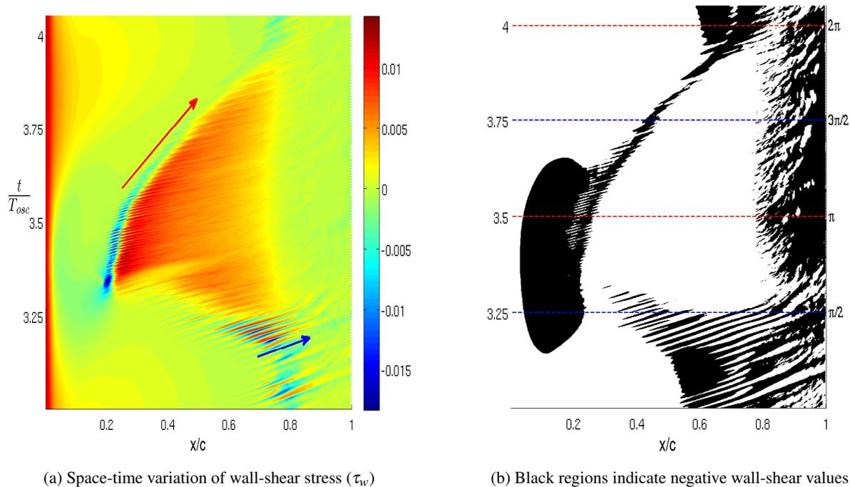
Figure 12: Space-time plot for the wall-shear values ( $\tau_w$ ) and separated flow regions. The values are obtained from the instantaneous flow averaged over the spanwise direction. Horizontal blue dashed lines in 12b represent the extremum positions of angle of attack, while the red dashed lines represent phases corresponding to mean angle of attack.
