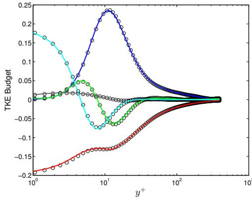
Figure 6: Comparison of turbulent kinetic energy budget normalized in inner units. Circles represent the DNS data from Moser *et al.* (1999) while the lines represent the values from the LES. The individual terms are color coded as: **Production**, **Dissipation**, **Viscous diffusion**, **Turbulent diffusion**, **Velocity-Pressure correlation**
