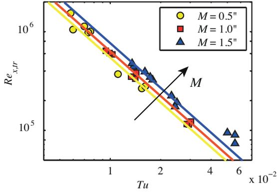
Figure 1. Transitional Reynolds number versus turbulence intensity for three different turbulence generating grids. Experimental data by Hislop (1940).
