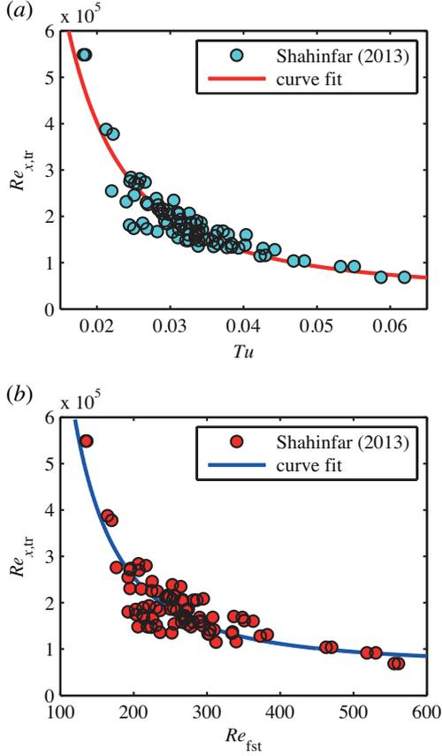
Figure 2. Transitional Reynolds number versus turbulence intensity in (a) and FST Reynolds number in (b). Experimental data from Shahinfar & Fransson (2013).
