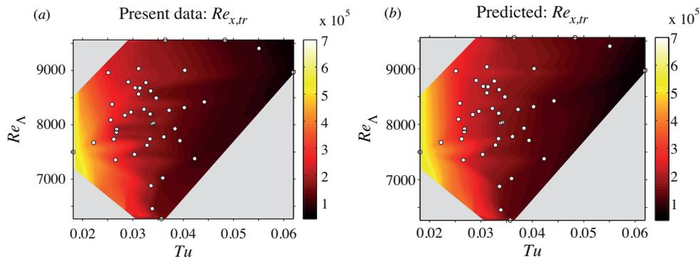
Figure 4. Transitional Reynolds number ( $Re_{x,tr}$ ) as a function of the Reynolds number based on the integral length scale ( $Re_{\Lambda}$ ) and  $Tu$  (both taken at the leading edge of the flat plate). (a) Experimental data. (b) Predicted data based on FST data at the leading edge of the flat plate.
