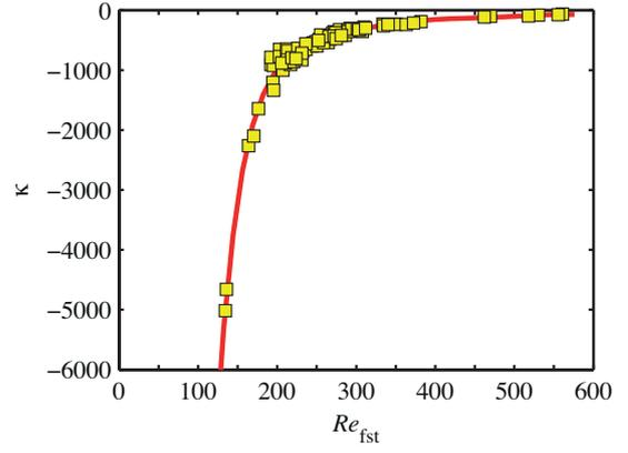
Figure 3. Weighting function ( $\kappa$ ) versus FST Reynolds number. Here, the model function, shown as a solid line, corresponds to a 6<sup>th</sup> order polynomial.
