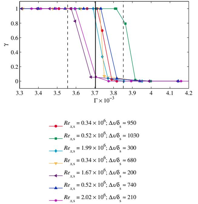
Figure 1. Intermittency  $\gamma$  of the near-wall velocity signal vs. the suction rate  $\Gamma$  for different suction start locations  $Re_{x,s}$  and streamwise evolution lengths  $\Delta x/\delta_s$ . Black solid line:  $\Gamma_{\text{crit}} = 3.70 \times 10^{-3}$  (Khapko *et al.*, 2016); Black dashed line:  $\pm 4\%$  deviation on  $\Gamma_{\text{crit}}$ .
