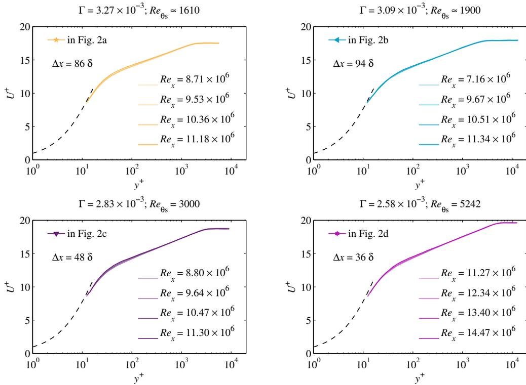
Figure 3. Inner-scaled mean velocity profiles for the four most downstream measurement locations for asymptotic cases in Fig. 2.  $\Delta x$  represents the streamwise distance between the most upstream and the most downstream boundary-layer profile shown in each graph. *Dashed line: Viscous sublayer as in eq. (1)*
