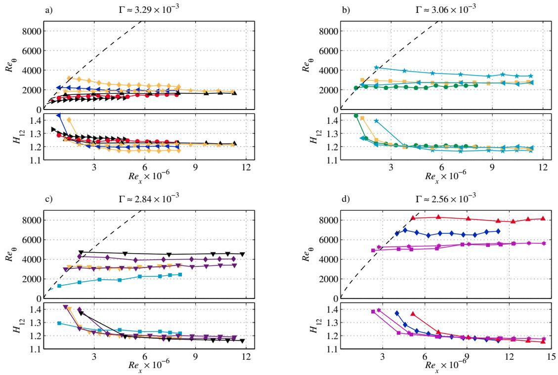
Figure 2. Influence of the boundary-layer thickness at the suction start location on the evolution of the boundary-layer momentum-thickness Reynolds number  $Re_\theta$  and shape factor  $H_{12}$ . *Dashed line:  $Re_\theta = f(Re_x)$  as in Nagib et al. (2007)*
