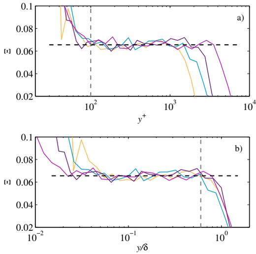
Figure 6. Indicator function  $\Xi$  vs. the inner scaled (a) and outer-scaled (b) wall-normal coordinate. *Black dashed line:*  $\Xi = 0.0656$ ; *Gray dashed line:* log-law bounds  $y^+ = 100$  and  $y/\delta = 0.6$
