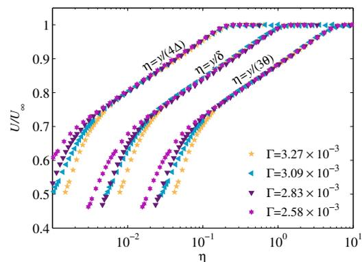
Figure 5. Outer-scaled asymptotic profiles at the most downstream measurement location, for three different choice of the outer length scale. The multiplicative coefficients of the length scales were chosen solely for illustration purposes. Symbols as in Fig. 2.
