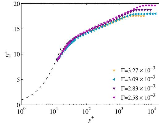
Figure 4. Inner-scaled asymptotic profiles at the most downstream measurement location. Symbols as in Fig. 2. Dashed line: Viscous sublayer as in eq. (1)
