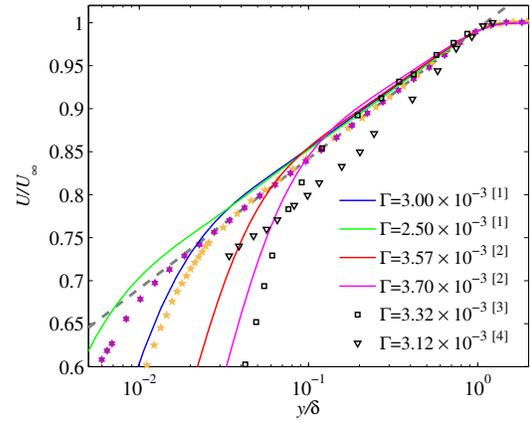
Figure 7. Comparison between present experiments and other experimental and numerical data. *Colored symbols:* current experiments, symbols as in Fig. 5; *Gray dashed line:* log-law as in eq. (7); [1]: LES simulations by Bobke *et al.* (2016); [2]: DNS simulation by Khapko *et al.* (2016); [3] Experiments by Kay (1948); [4]: Experiments by Tennekes (1964) (run 2-312;  $x = 878$  mm).
