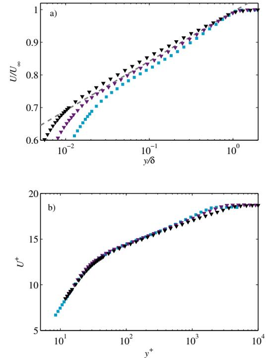
Figure 8. Inner- (a) and outer- (b) scaled mean velocity profiles for the most downstream location of three cases with  $\Gamma \approx 2.83 \times 10^{-3}$ . Symbols as in Fig. 2c. *Gray dashed line:* log-law as in eq. (7).
