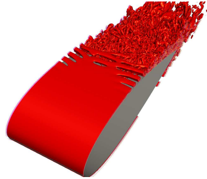
Figure 4: Isosurface of Q = 2500 \text{ s}^{-2} at AOA = 5^\circ .
