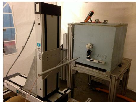
**Figure 1** Jet facility, hot-wire probe and 3-axis traversing mechanism. For practical reasons, flow blockage due to the traversing system is difficult to avoid. This has been countered by placing the probe on a lengthy, but stable, extension arm to increase the distance between traversing system and probe.
