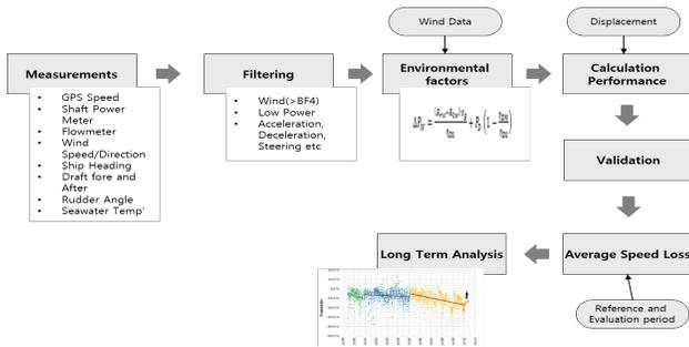
Fig. 6 Measurement and analysis process of ISO19030
