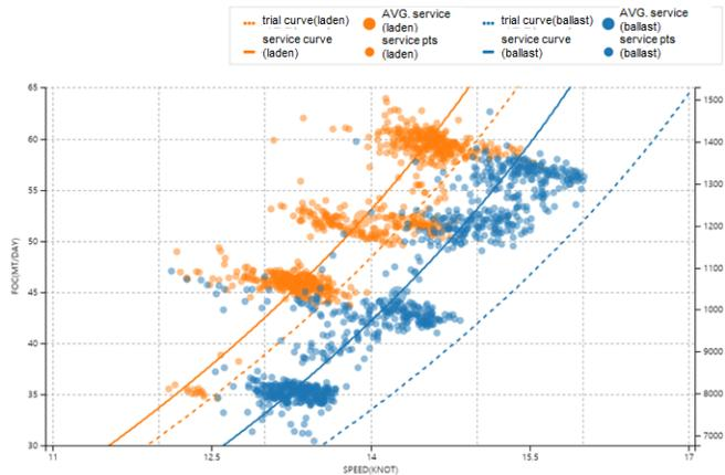
Fig. 9 PV analysis result during 8 months after drydocking
