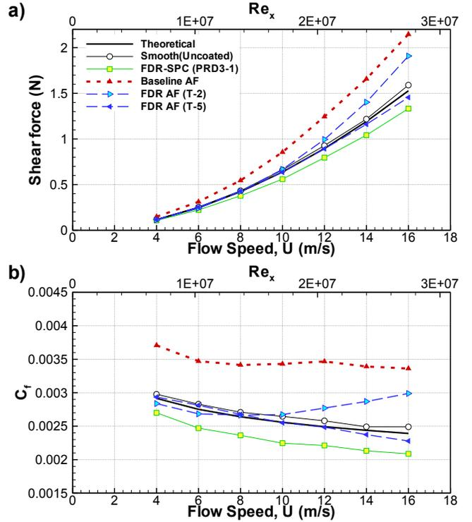
Fig. 2 Comparison of frictional drag in high Reynolds number flow for FDR-SPC and FDR AF coatings
