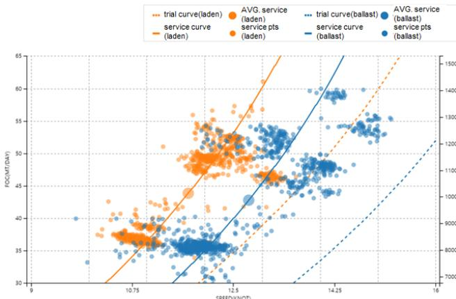
Fig. 8 PV analysis result during 8 months before drydocking
