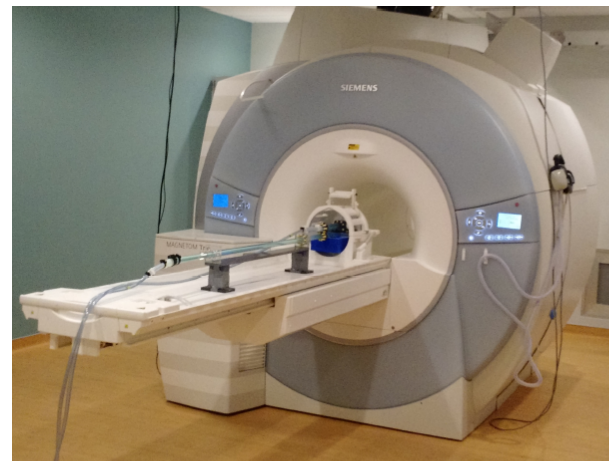
Fig. 2. The 3 Tesla Siemens MRI scanner used for the MRV measurements, with the model inserted in the head coil.
