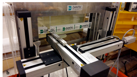
Figure 1. Computer-controlled three-axis traversing system (a) the design schematic (b) the actual unit.
