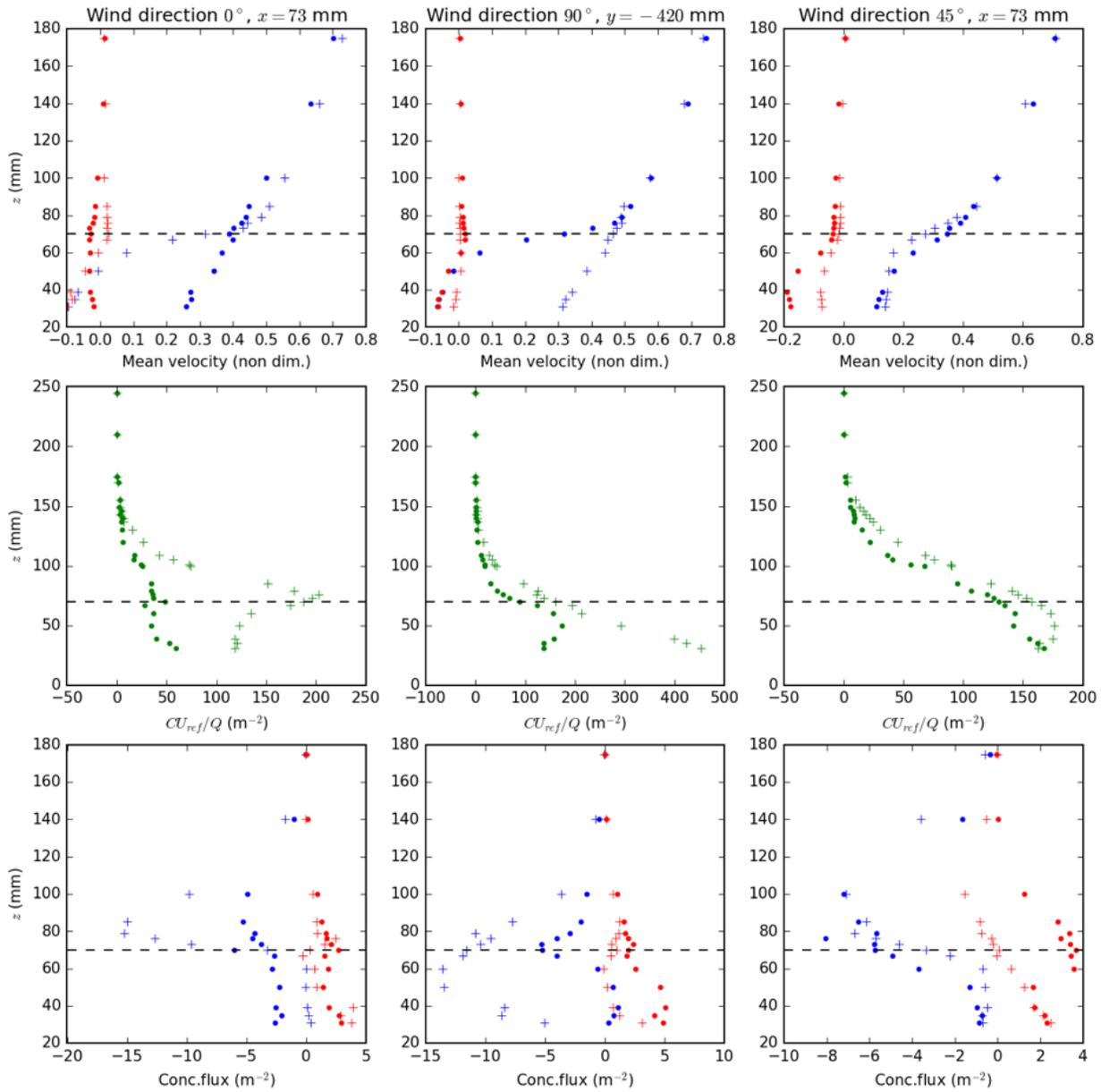
Figure 3. Selected velocity, concentration and concentration flux profiles. Blue =  $U/U_{ref}$  and  $uc/Q$ ; red =  $V/U_{ref}$  and  $vc/Q$ ; '+' represent profiles at  $y = 0$  ( $0^\circ$ ),  $x = 3$  mm ( $90^\circ$ ),  $y = -315$  mm ( $45^\circ$ ); '.' represents profiles at  $y = -105$  mm ( $0^\circ$ ),  $x = -67$  mm ( $90^\circ$ ),  $y = -420$  mm ( $45^\circ$ )
