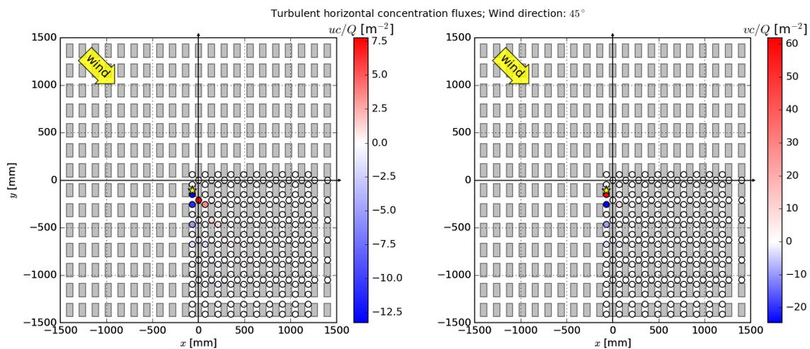
Figure 8. Horizontal turbulent mass fluxes within the canopy for the  $45^\circ$  case.
