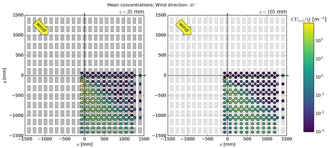
Figure 5. Non dimensional concentrations within (left) and above (right) the canopy for the  $45^\circ$  case.
