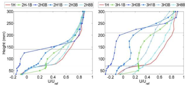
Figure 11. Selected vertical velocity profiles at various distances downwind (0B = street below tall building, 1B = 1 street downwind 0B, and so on).
