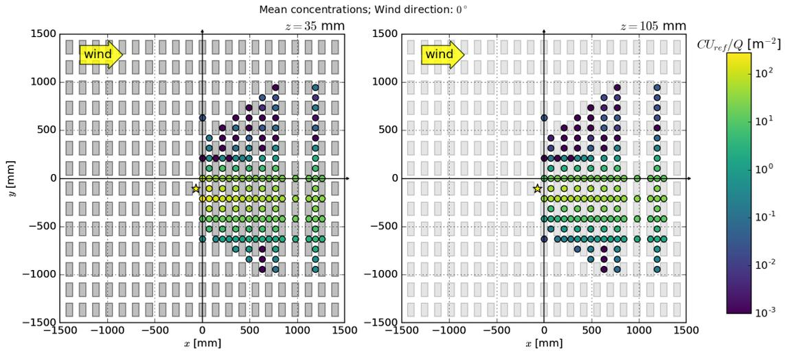
Figure 4. Non dimensional concentrations within (left) and above (right) the canopy for the  $0^\circ$  case.
