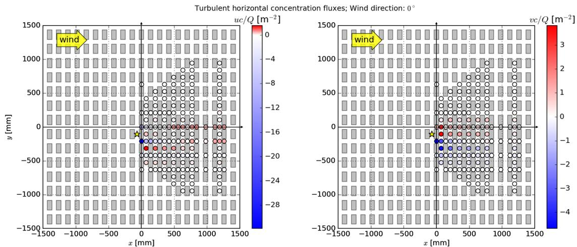
Figure 7. Horizontal turbulent mass fluxes within the canopy for the  $0^\circ$  case.
