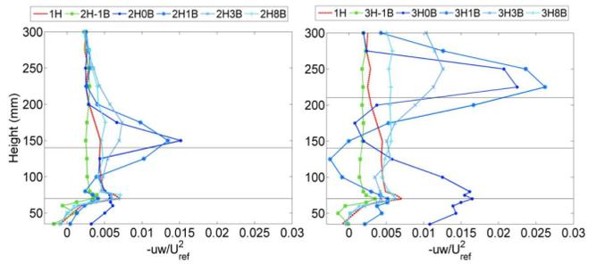
Figure 12. Selected Reynolds stress profiles at various distances downwind (0B = street below tall building, 1B = 1 street downwind 0B, and so on).
