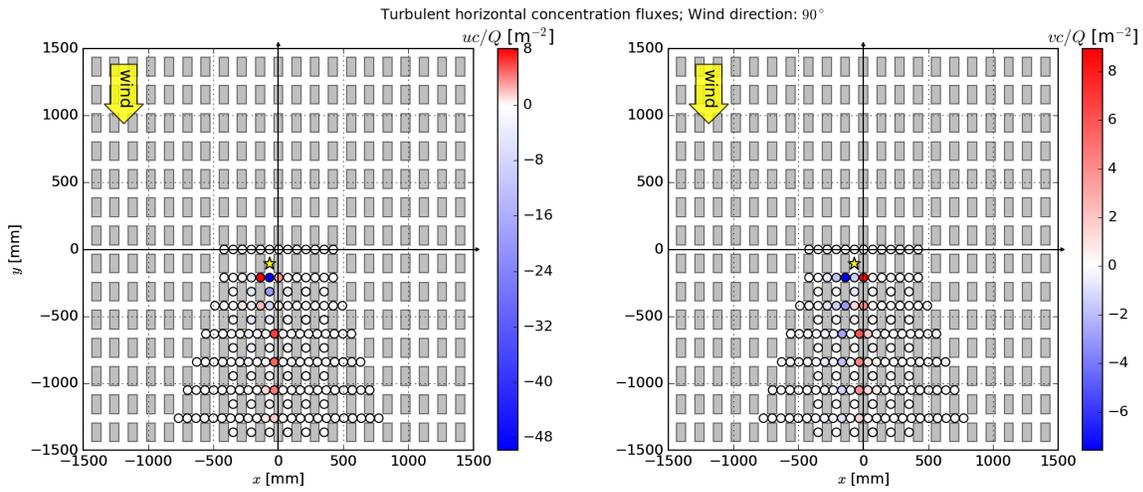
Figure 9. Horizontal turbulent mass fluxes within the canopy for the 90° case.
