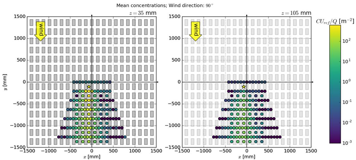
Figure 6. Non dimensional concentrations within (left) and above (right) the canopy for the  $90^\circ$  case.
