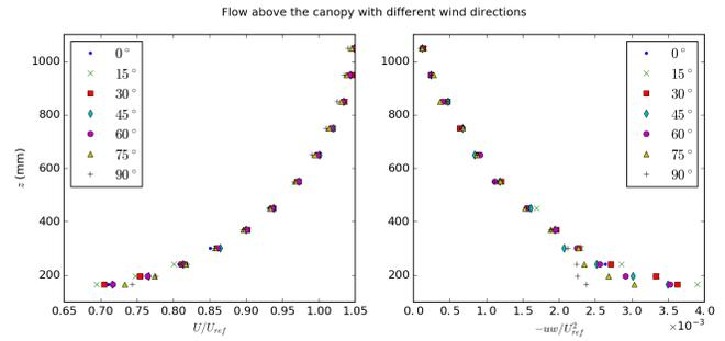
Figure 2. Spanwise averaged profiles of velocity and vertical momentum fluxes above the canopy (normalised using the free-stream velocity) with different wind directions.
