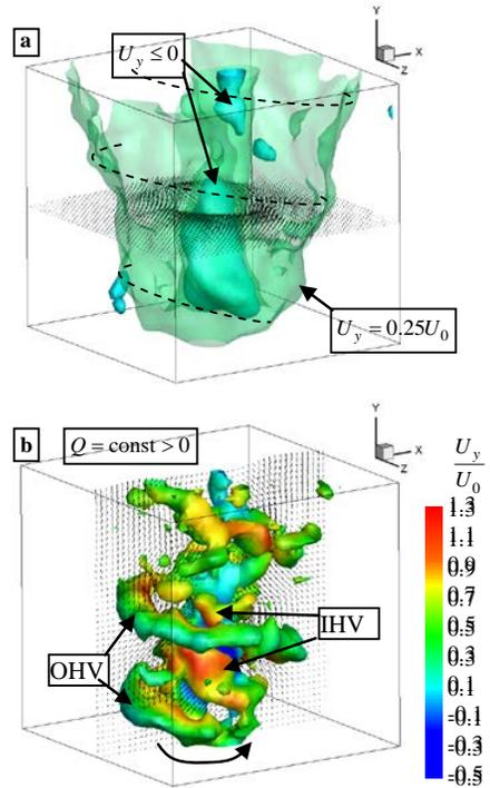
Figure 7. The instantaneous velocity data for a high-swirl jet ( $S = 1.0$ ,  $Re = 8\,900$ , 3D PIV)
