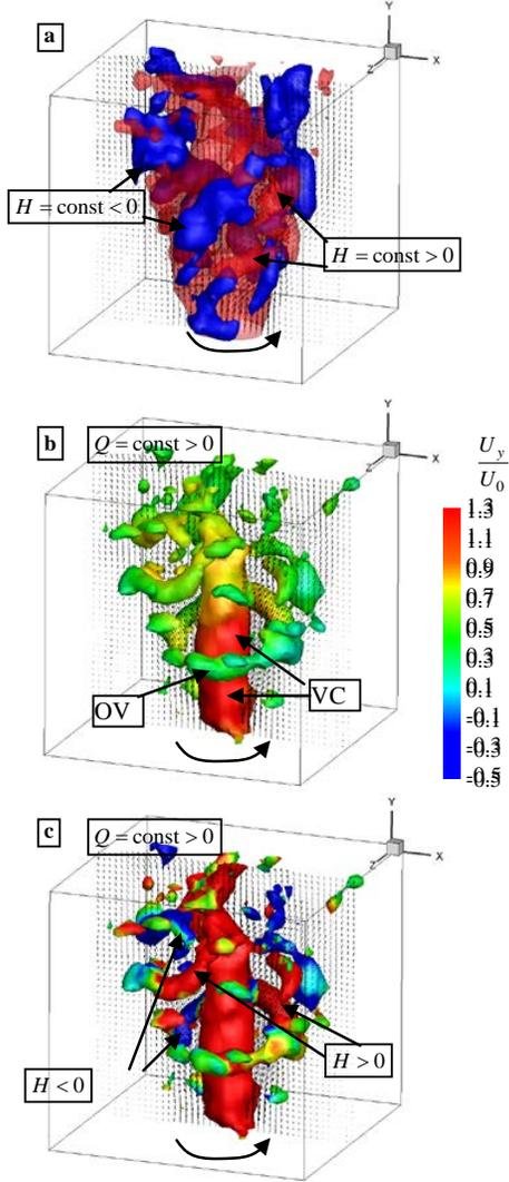
Fig. 8. The instantaneous velocity and vortical structures for a low-swirl jet ( $S = 0.41$ ,  $Re = 8\,900$ , 3D PIV). (a) - Positive (red) and negative (blue) helicity iso-surfaces; (b) and (c) -  $Q$  criterion colored by the axial velocity and helicity, respectively.
