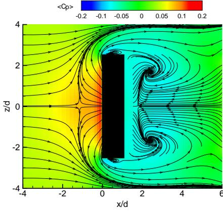
Figure 4. Horseshoe vortex in front of the first-row obstacle in the central column, visualized using time-averaged pressure coefficient and streamlines in the  $x$ - $z$  plane at elevation  $y/d = 0.2$ .
