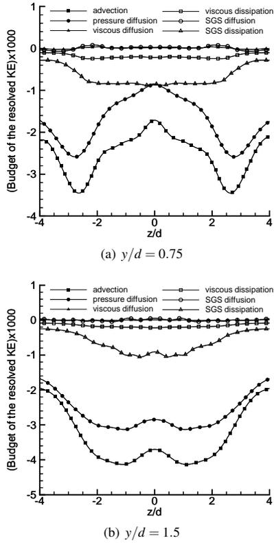
Figure 7. Budget of the time-averaged resolved kinetic energy ( $k_r$ ) at  $x/d = 35.3$  within  $-4 < z/d < 4$ , at two different elevations. All the quantities shown in the figures have been non-dimensionalized using  $U_\infty^3/d$ .
