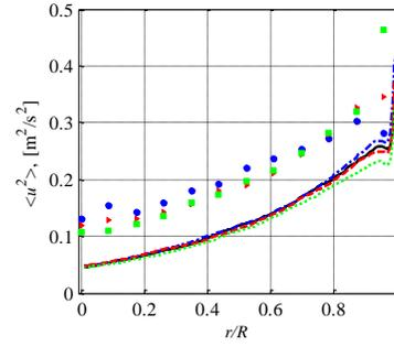
Figure 3. Streamwise turbulent fluctuations of liquid and solid phases. Legends are the same as Fig.2.
