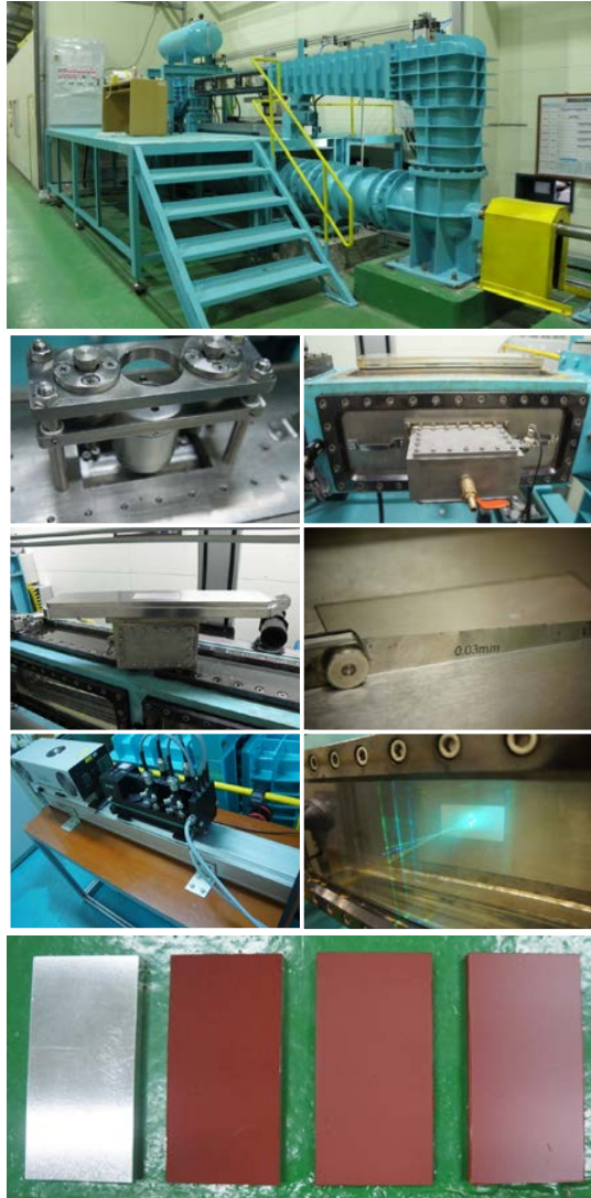
Figure 4 Photos of the high-speed water tunnel, flush-mounted balance and the samples of FDR-SPC and FDR-AF coatings
