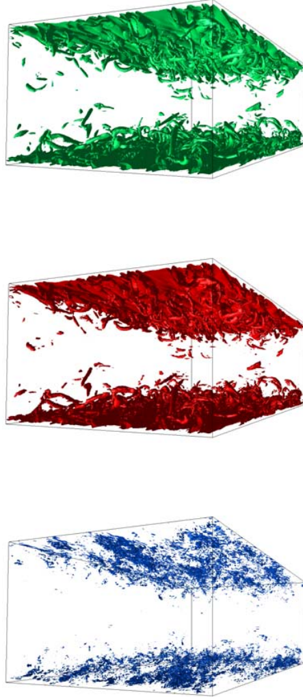
Figure 1. Visualization of total vorticity \boldsymbol{\omega}^+ (top), coherent vorticity \boldsymbol{\omega}_c^+ (middle) and incoherent vorticity \boldsymbol{\omega}_i^+ (bottom). Isosurfaces |\boldsymbol{\omega}^+| = |\boldsymbol{\omega}_c^+| = 10.0 and |\boldsymbol{\omega}_i^+| = 3.5 are presented, respectively.
