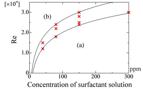
Figure 9. Profile of meandering conditions. (a) stability area and (b) instability area.
