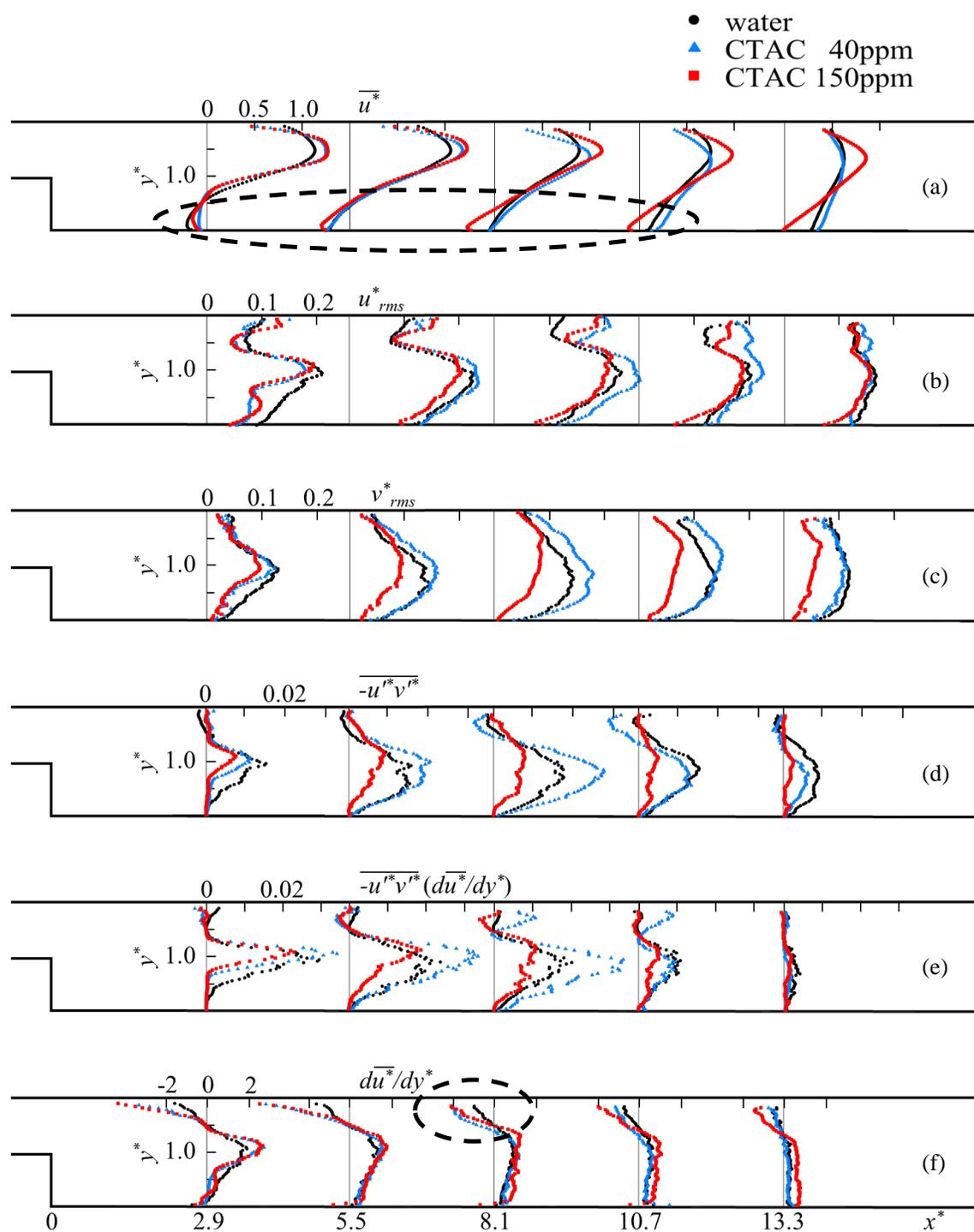
Figure 3. Turbulence statistics profiles at  $Re = 1.5 \times 10^4$ . (a) Mean streamwise velocity, (b) Root mean square of streamwise velocity fluctuations, (c) Root mean square of wall-normal velocity fluctuations, (d) Reynolds shear stress, (e) Turbulence production and (f) Mean streamwise velocity gradient.
