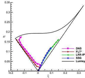
Figure 9 Reynolds-stress invariants of turbulence model and DNS.
