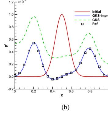
Figure 1 Propagation of the pressure perturbation in gravitational field.
