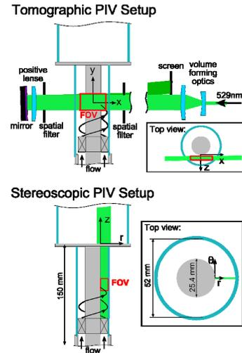
Figure 2. Diagnostic setups and fields of view for volumetric (top) and planar (bottom) PIV measurements.
