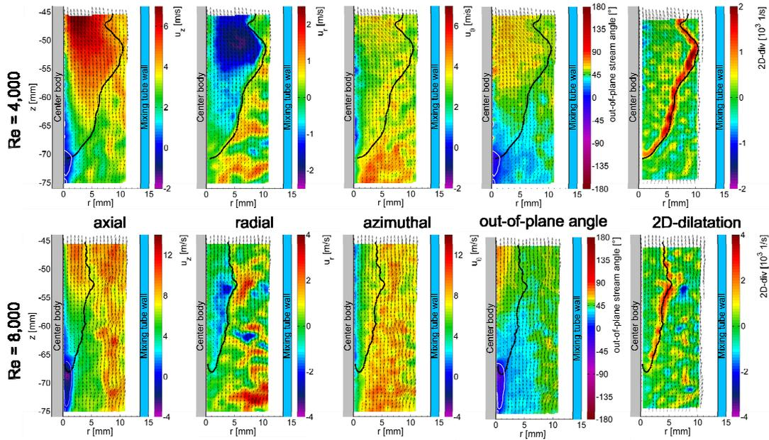
Figure 7. Radial-axial slices showing all three velocity components, the out-of-plane angle (angle between the streamwise direction and the horizontal plane) and the in-plane dilatation. Top row:  $Re_h = 4,000$ . Bottom row:  $Re_h = 8,000$ . Black line: Flame front. Every third velocity vector is plotted.
