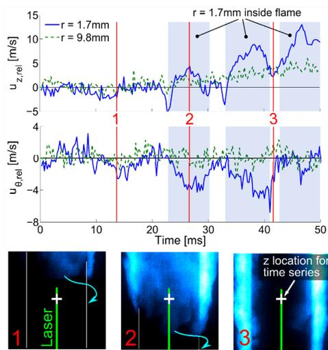
Figure 8. Relative axial (top) and azimuthal (bottom) velocity traces over time at axial location  $z = -49.2$  mm and two radial locations  $r = 1.7$  mm (close to center body wall) and  $r = 9.8$  mm (core flow). Chemiluminescence images show flame at time instants 1, 2 and 3.  $Re_h = 8,000$ .
