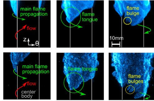
Figure 4. Chemiluminescence images taken from a movie sequence showing the flame inside the mixing tube during a methane-air (top row) and hydrogen-methane-air flashback (bottom row) at three instants in time.
