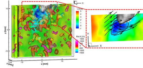
Figure 6. Flow field upstream of the flame front (grey surface) during a methane-air flashback. Flooded contour shows axial velocity. Black solid line marks 0 m/s axial velocity. Vortical structures are visualized by an iso-surface of  $\lambda_2$  and colored by the x-component of vorticity. Black solid lines with arrows in zoomed view are streamlines.
