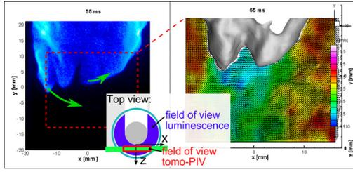
Figure 5. Simultaneous high-speed tomographic PIV (right, axial velocity field) with 3D-flame surface (grey) and chemiluminescence imaging (left) showing a methane-air flame flashback. Note the different depths in the field of view.
