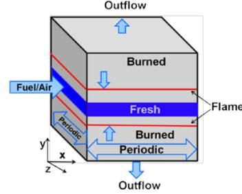
Figure 1. Configuration diagram of the DNS of  $H_2$ /air premixed turbulent combustion
