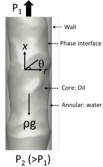
Figure 1. Schematic diagram of core-annular flow
