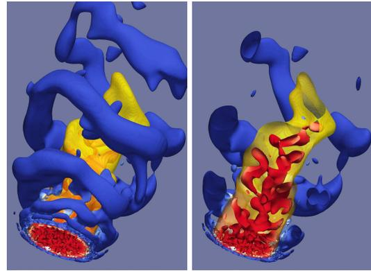
Figure 10. WENO-OPT /  $F = 6 +$  sgs ( $OP_2$ ). Q-criterion colored by  $Y_{CH_4}$  (left), and inner structure of the flow (right). The flame surface is materialized by the  $c = 0.5$  iso-surface (mainly yellow), colored by the reaction rate  $\dot{\omega}_{CH_4}$ .
