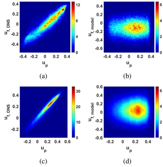
Figure 8: Contours of joint PDF of instantaneous velocities in the shear regime at  $\tau_j = 7$ . (above):  $St = 1$ , (below):  $St = 0.1$
