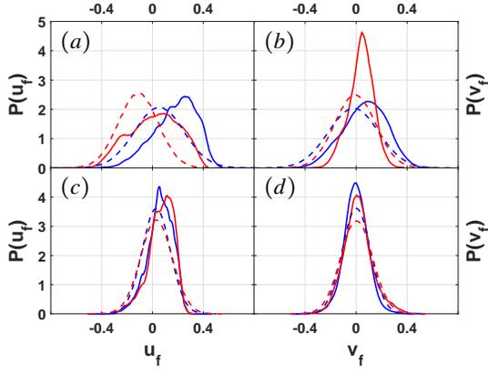
Figure 7: PDF of instantaneous velocities at location of shear layer. (above):  $\tau_j = 7$ , (below):  $\tau_j = 43$  (—)  $St = 0.1$ , *DNS*; (- - -)  $St = 0.1$ , *model*; (—)  $St = 1$ , *DNS*; (- - -)  $St = 1$ , *model*.
