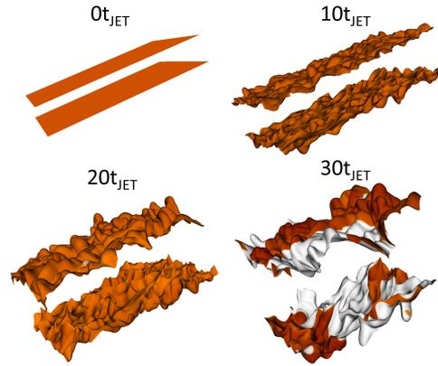
Figure 4. Evolution of  $Z_{ST}$  surface with time. Surface is coloured by temperature threshold. Orange colour indicates non-burning, white indicates burning ( $T > 1500$  K).
