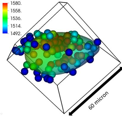
Figure 3. Example of particle ensemble for an ignition kernel. The surface is  $HRR_T$  coloured by temperature. The spheres are Lagrangian tracer particles coloured by temperature to the same colour scale.
