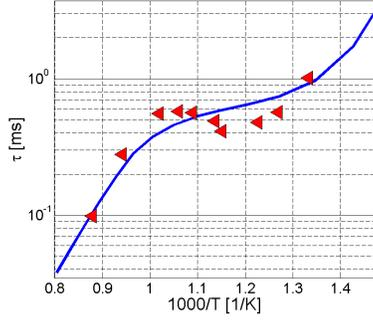
Figure 2. Validation of ignition delay times. Data points are experimentally values from Ciezki & Adomeit (1993), the blue line is obtained from the program SENKIN, developed by Lutz *et al.* (2002), using the rates detailed in table 1.
